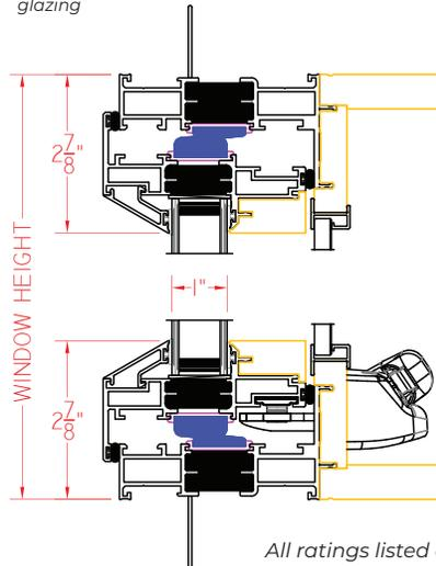
Shown with narrow sightline, nailing fin and traditional, sloped exterior glazing
