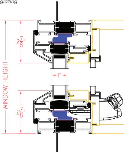
Shown with nailing fin and traditional, sloped exterior glazing
