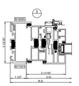
SERIES M600 CONFIGURATION FIXED OVER AWNING INSTALLATION METHOD RECEPTOR AND SUBSILL
