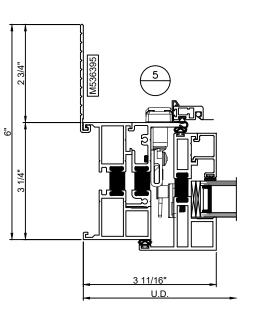
SERIES M600 CONFIGURATION FIXED OVER AWNING INTERIOR ANCHOR STRAP
