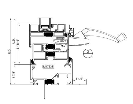
SERIES M600 CONFIGURATION FIXED OVER AWNING INSTALLATION METHOD RECEPTOR AND SUBSILL W/ FLASHING FLANGE
