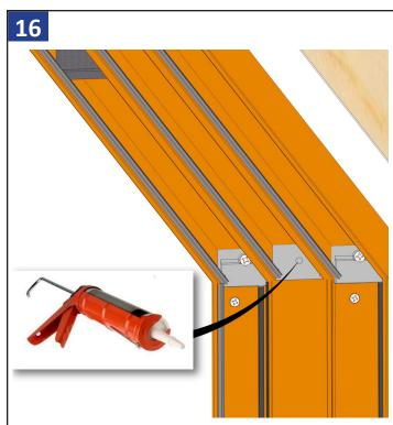
Fill the corner keys with sealant through the small injection port until there is ooze out.
