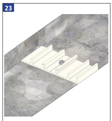
Install anchor clips as shown above and apply sealant over fastener heads.
