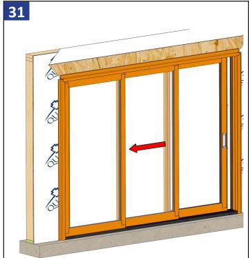
Slide the exterior most panel into the jamb.
