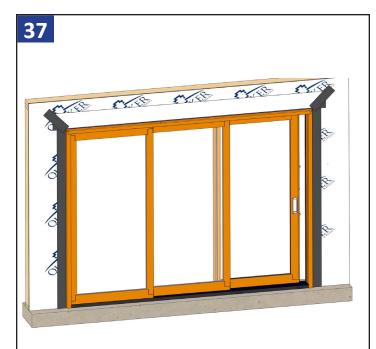
Unfold the house wrap top flap and tape the angled seams as shown.
