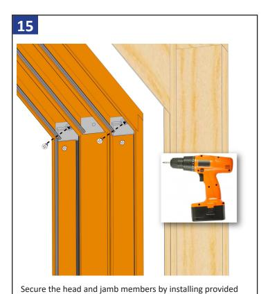
screws into the two screw bosses in each corner key.
