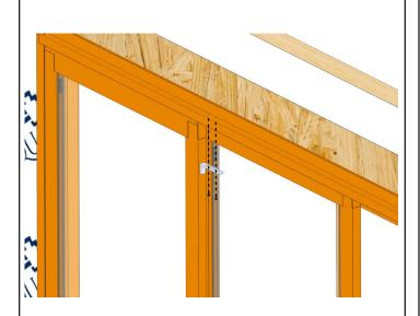
With the fixed panel properly shimmed, install the angle bracket in the head track with provided screws and lock washers to secure the panel in place.
