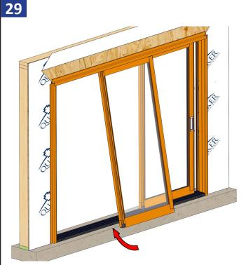
Repeat for the middle panel, setting it into the middle tracks in the head and sill.
