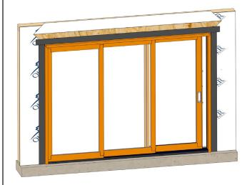
Apply a 3/8" sealant bead to the top exterior edge of door frame before installing the drip cap.
