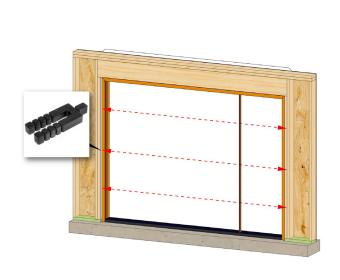
Check that the door frame is not bowed at jambs or head, a string line may be required. The jamb cover can be used to ensure equal spacing between the sill and head. Adjust shims as needed until measurements are within 1/8". Shim at sides and at lock locations as required.
