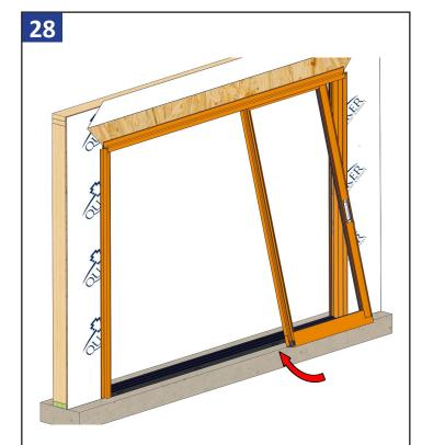
From the exterior, install the most interior panel by tilting the top into the inner most head track and setting the bottom of the panel in the inner most groove in the sill track.
