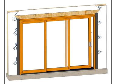
Apply flashing tape at the sides of the door as shown. Smooth using a J-roller. Extend tape a minimum of 2" past door frame, but not more than the thickness of the flashing tape.
