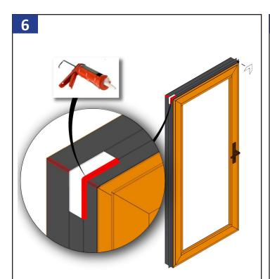
Install the two top foam corner key gaskets over the exterior side of the positioning fin corner gaps. Seal the exterior corners where the gasket meets the positioning fin as shown above.
