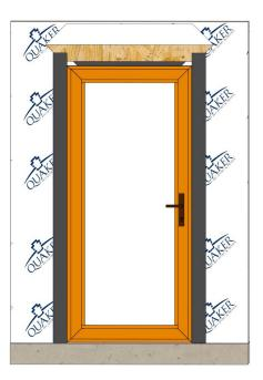
Cut two pieces of flashing tape for jamb flashing extending 1" above the head positioning fin. Apply flashing tape and smooth using J-roller.
