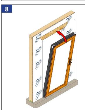
Center the door in rough opening, lifting and setting the bottom of the door in first, then tilting into place.. Verify for squeeze out of sealant all along positioning fin.
