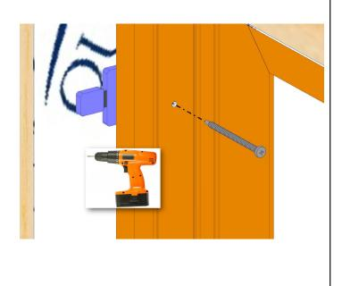
Drill a pilot hole through the jamb's walls per anchorage calculations. *Quaker Window Products does not supply or claim liability for anchorage/fastener calculations. It is the installer/client's responsibility for structural adequacy of the anchorage and fasteners*. Typically, a #12 screw 6" from the top and bottom and 16" on center thereafter. Install and fasten the door unit in place using fasteners by others per anchorage calculations.
