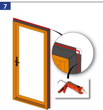
Apply a continuous 3/8" bead of sealant around the perimeter of the interior side of the positioning fin as shown.
