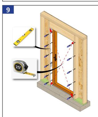
Square, level, and plumb unit in the rough opening by applying shims as needed. Shim behind all hinges and lock points, do not over shim, do not shim at the head.
