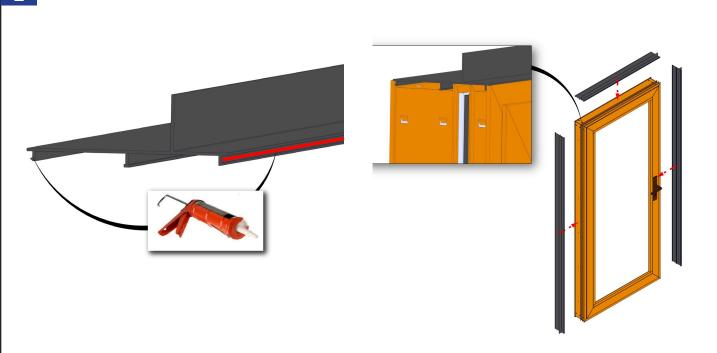
Apply sealant on the exterior legs of the positioning fin as shown above, and install the positioning fin into place with the short side of the flange facing the exterior.
