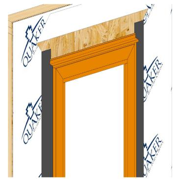
Place the drip cap the full width in sealant as shown.
