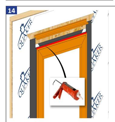
Apply a 3/8" bead of sealant to the top exterior edge of door frame before installing the drip cap as shown.
