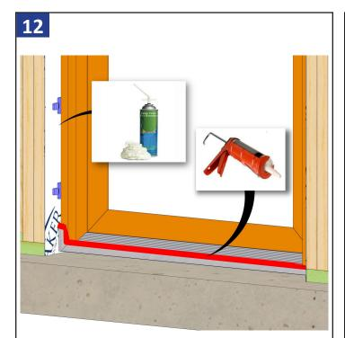
Apply a bead of sealant to fill the gap between the sill pan flashing system and the door unit. Make sure to seal all the way up both ends of the corner mold against the door. Insulate around the entire perimeter of the door.
