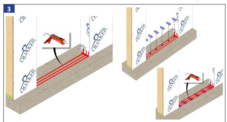
Apply three continuous 3/8" beads of sealant on the sill where the pan flashing will set. Also generously apply sealant along the bottom corners of the rough opening. Set shims in the bed of sealant and apply more sealant over the top of the shims.
