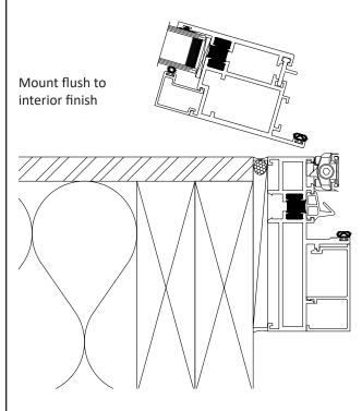
For inswing units where full panel operation is desired, install the unit flush with interior finish surface of wall.
