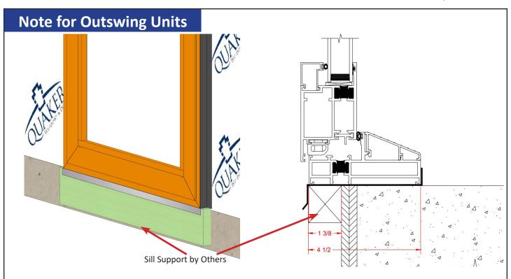
The sill must be supported the full width and depth of unit. For installations where the unit does not have full sill support, additional support must be installed under the sill.
