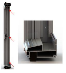
Drill pilot holes (if necessary) in the new window frame. Plan ahead for all holes especially the top of jamb. Make sure top pilot hole will not be in the same locations as the weight pulleys. Use a 1/8" drill, and minimum of 3 holes per jamb. Place holes in center of inside balancer track minimum of 3" from corners, and one in center of the check rail. Tilt the bottom sash in or remove it to place the center pilot hole.
