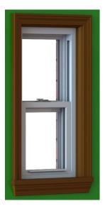
Insulate between the window frame and the rough opening using minimally expanding window and door spray foam or fiberglass insulation. Operate window unit to ensure proper operation. Sash will not operate correctly if window is out of square, over-shimmed or over-insulated. Allow foam to fully cure before installing interior trim. Install interior stops that were remove earlier or cut new stops.
