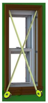
Check for plumb, level, square and window operation. Make any necessary adjustments to shims and finish installing frame screws. Raise bottom sash to install bottom screws, and tilt bottom sash in to install center screws.
