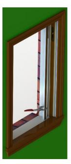
Remove the jamb and head parting stops (if applicable) by pulling or prying them out of the frame.
