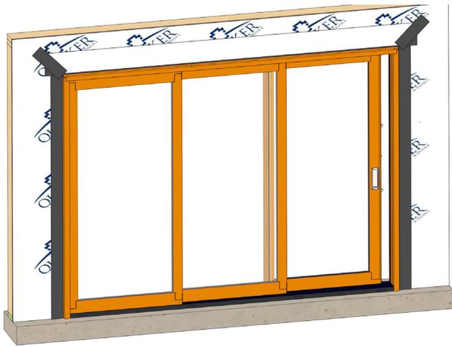
Unfold the house wrap top flap and tape the angled seams as shown.
