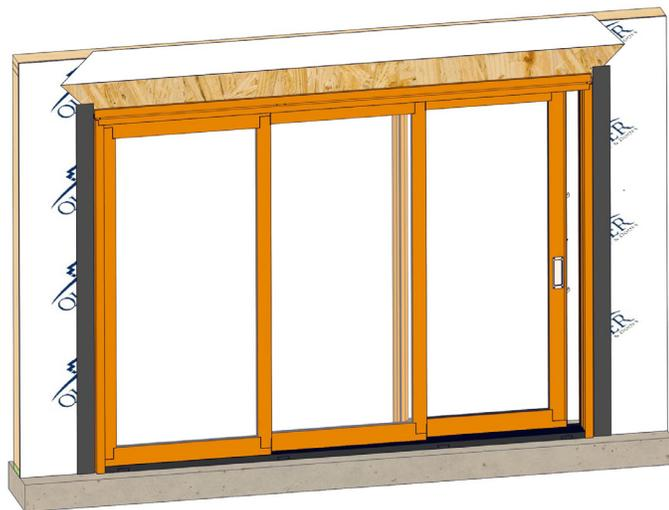
Apply flashing tape at the sides of the door as shown. Smooth using a J-roller. Extend tape a minimum of 2" past door frame, but not more than the thickness of the flashing tape.
