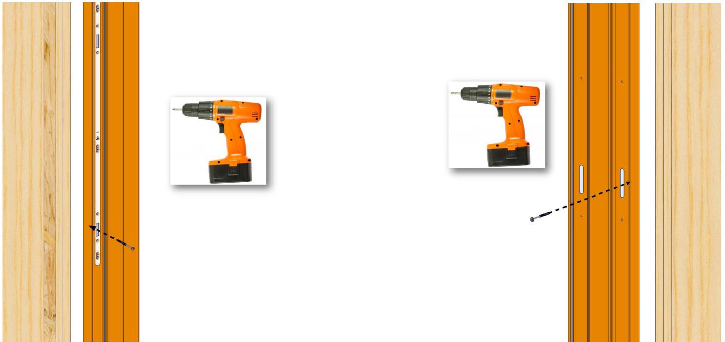
In the lower slotted hole in each jamb, drill a hole and loosely fasten the jamb to the wall framing. The fastener needs to be loose for squaring and plumbing of the frame.
