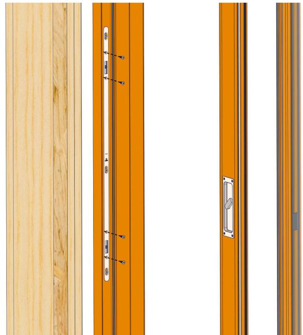
Adjust the strike plate up or down as needed for the lock to properly engage. Secure the strike plate and install the 4 additional screws.
