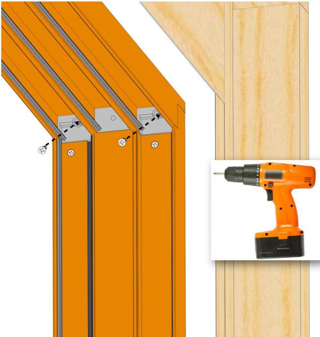
Secure the head and jamb members by installing provided screws into the two screw bosses in each corner key.
