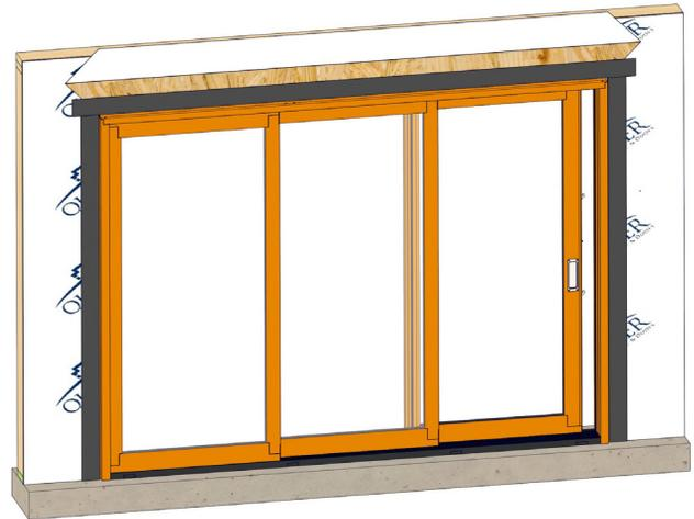
Apply a 3/8" sealant bead to the top exterior edge of door frame before installing the drip cap. Apply flashing tape over the drip cap leg, overlapping the side flashing as shown. Smooth using a J-roller.
