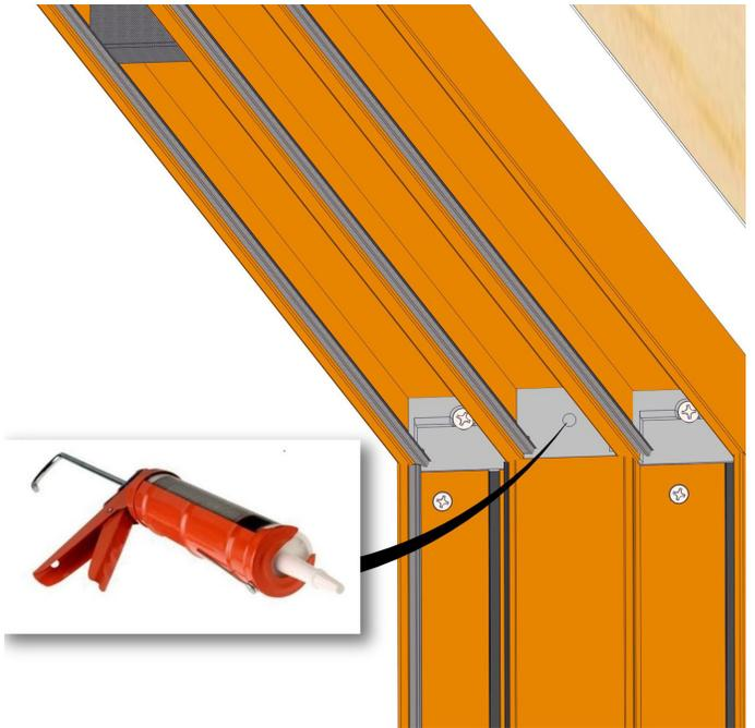
Fill the corner keys with sealant through the small injection port until there is ooze out.
