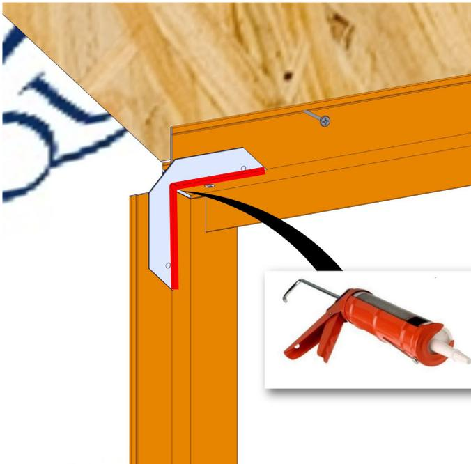
Apply the 2 corner gaskets to each corner and apply sealant as shown above.
