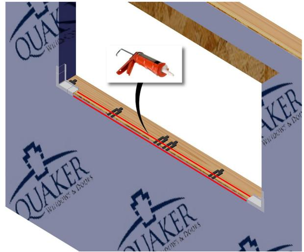
Apply a continuous beads of sealant on the sill and exterior wall face between the corners as shown above.
