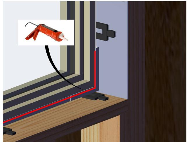
Apply a bead of sealant to fill the gap between the sill pan flashing system and the window unit. Make sure to seal all the way up both ends of the corner mold against the window also.
