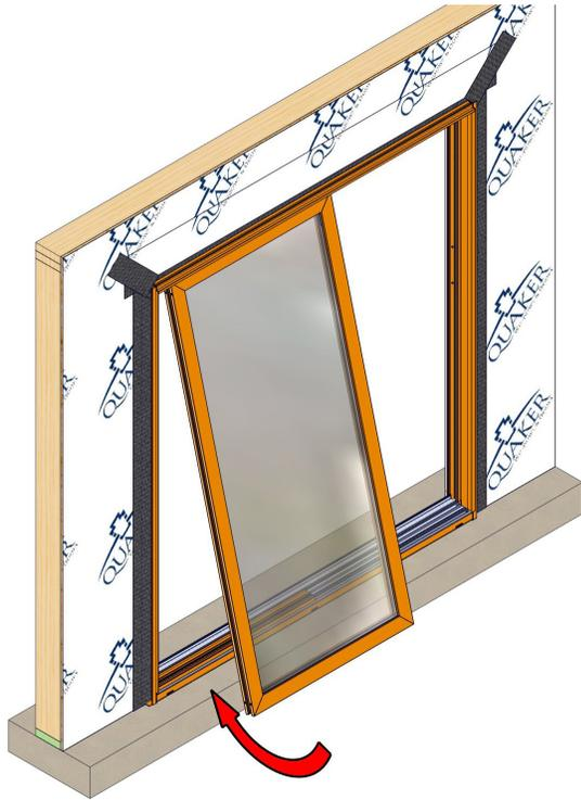
Angle the fixed panel with the top inserted into the head track, and then lift and set the bottom of the panel on the fixed panel extrusion in the sill.
