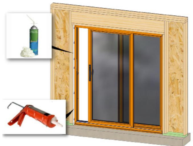
Fill interior 1/3 of cavity using low expanding foam or backer rod and apply sealant continuously around entire perimeter of opening.
