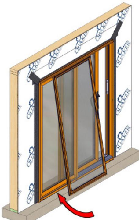
Angle the screen panel with the top inserted into the head track, and then lift and set the bottom rollers on the roller track. Adjust rollers as needed to insure the panel is level, square, and slides smoothly.
