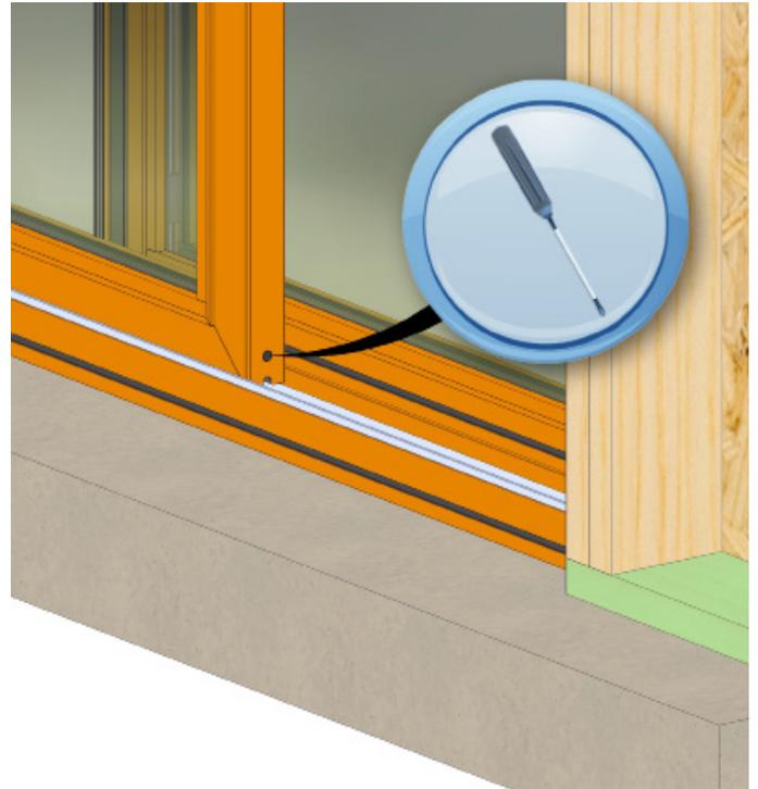
From the interior, angle the active panel with the top inserted into the head track, and then lift and set the bottom rollers on the roller track.
