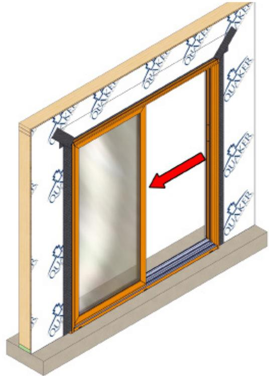
Slide the panel tight against the frame keeping the panel flush with the fixed panel extrusion in the sill.
