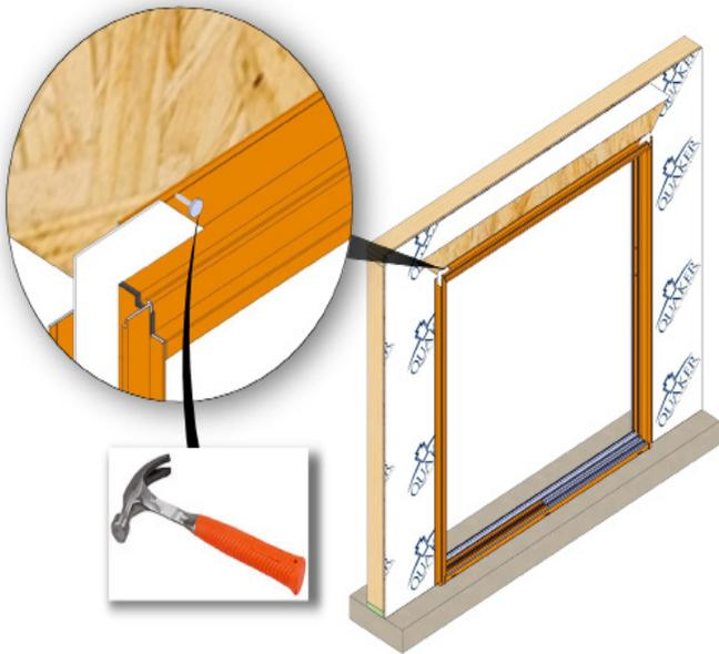
Temporarily tack the door into place using 2" galvanized roofing nails through the pre-punched holes on one top corner of the nailing flange.
