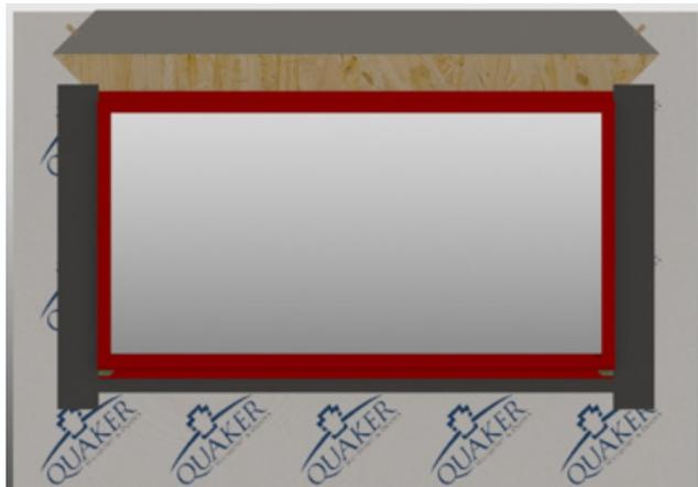
Cut two pieces of flashing tape for jamb flashing extending 1" above flashing flange system head flange and 4" to 6" below bottom edge of sill flashing. Remove release paper and press tightly along sides of window frame.
