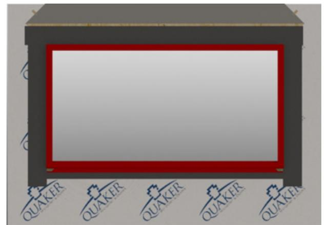
Cut a piece of flashing tape for the head flashing, which extends beyond outer edges of jamb flashings. Remove release paper and install completely covering mounting flange and adhering to exposed sheathing or framing members.
