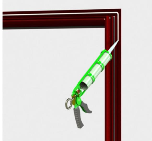
Apply a 3/8" diameter bead of sealant along the interior side of the flashing flange. Bead must run continuously around both sides and across the head.
