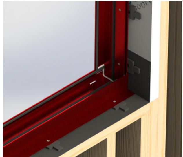
Apply sealant in installation holes or on screws. Fasten the flange fin system to framing with screws by others per shop drawings or anchorage calculations.
