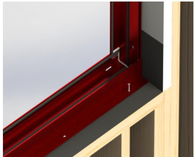
Center and set the flashing flange system into the rough opening. Pulling the system tight towards the interior making sure flashing flange is tight against the WRB. Temporarily screw the window into place using a screw through the pre-drilled pilot holes on the sub-sill anchor flange. **Do not** screw through flashing flange.
